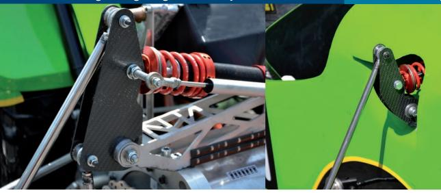
Fibre-reinforced plastic/metal composite for use in vehicle construction
