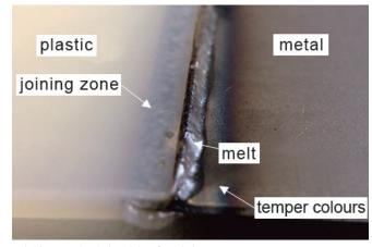
Hybrid composites in butt joints for tubular components
